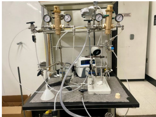
Rapid small-scale column test experimental setup.
